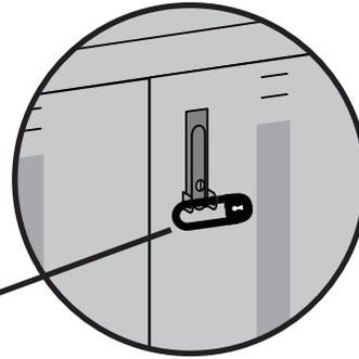
For added security, each door features hasps to hold your own padlock (maximum shackle dia 5/16"; minimum shackle height 2"). When installed, your padlock restricts access to the handle so the unit can't be opened.
