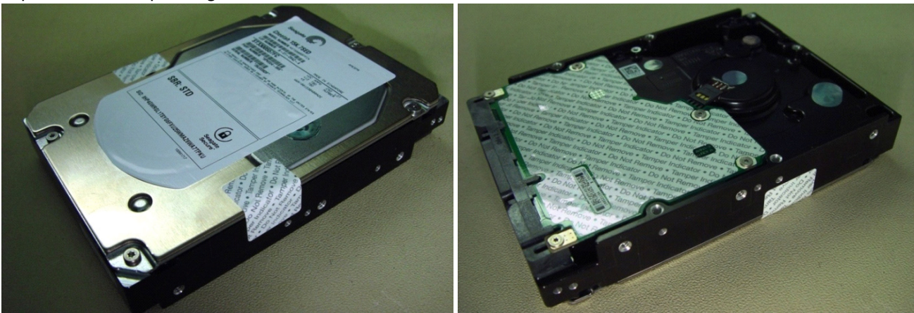
Figure 5. Example of FIPS tamper evidence labels.
