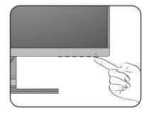
Turn on the computer too, and select an input source by the OSD control keys. The displayed input icons vary depending on the available video inputs of the purchased model.
