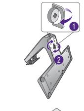
Orient and align the stand arm with the monitor, then push them together until they click and lock into place.
