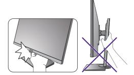
• If the monitor has been rotated to portrait mode and height adjustment is desired, you should be noted that the wide screen will keep the monitor from being lowered to its minimum height.
