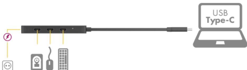
**Note:** In order to power and charge your connected laptop, its USB Type-C™ port must support USB Power Delivery or Thunderbolt 3™.
